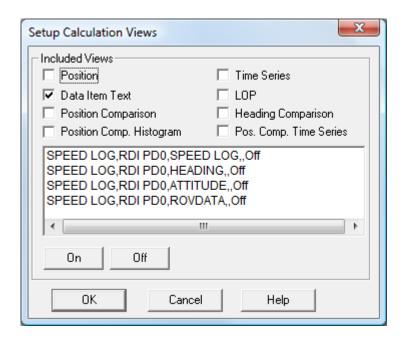
Select the *Data Item Text* checkbox, highlight the SPEED LOG item and then click the *On* button. Exit with *OK*. The speed log data can then be monitored in this Calculation window, as shown below.
